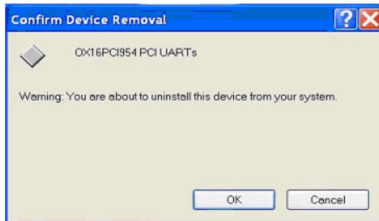
6. Wait for the removal to finish then go back to the System Properties window, click Multi-function adapters, and select OXmPCI954 PCI bridge.
