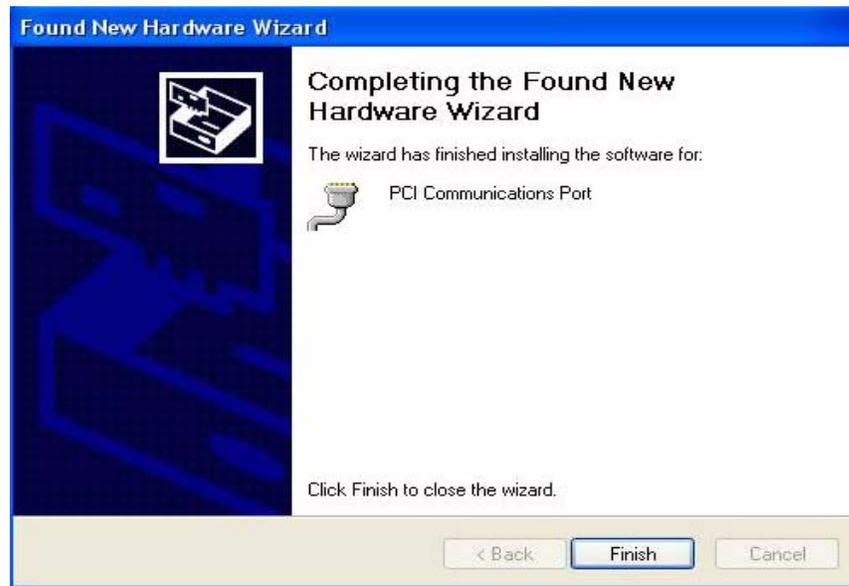
Windows will then search, find, and install driver for the 16 PCI communications ports automatically. Wait for the process to complete.
