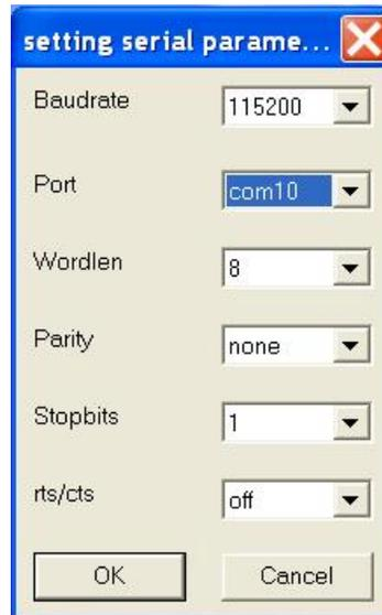
4. Start another sertest. Repeat step 1 through 3 to open the other COM port. In one window click Log, and in the other window, click Play. The following screen shows a file transferring between COM10 and COM11.
